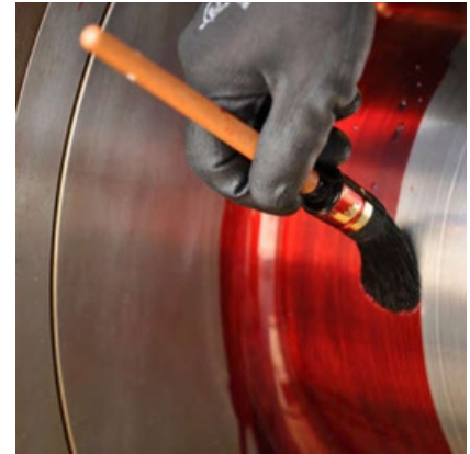
DYE PENETRANT TESTING
